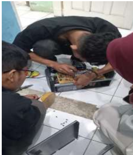
Gambar 3. 2 Pergantian baterai UPS
